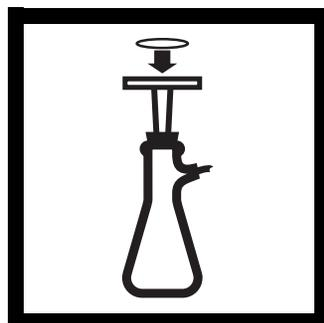
**3.** Set up the Membrane Filter Apparatus; see *Preparing Materials* on page 2. With sterile forceps, place a membrane filter, grid side up, into the assembly.
