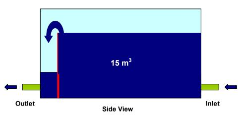
Figure 7: Water Reservoir with Minimum Volume of Water in Storage = 15m<sup>3</sup>
