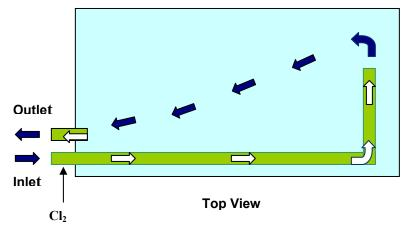
Figure 4: Water Reservoir with Mixing and Short Circuiting (F<sub>sc</sub> = 0.1)
