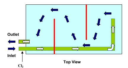
Adding baffles can be done at a reasonable cost by hanging sheets of plastic from stainless steel hangers and using stainless steel angle iron to hold the plastic tight to the wall and floor. It is very important that the plastic is approved for use in a potable water situation. NSF certification is required on the plastic, but these products are available.
