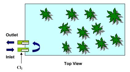
As an absolute minimum, the distance from the inlet to the outlet pipes should be maximized as illustrated in Figure 9. Although short circuiting is still significant, this configuration is a big improvement over the adjacent inlet and outlet pipe scenario.
